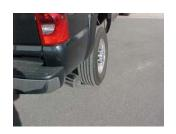
INSTALL STAINLESS STEEL TIP. CLAMP DOWN. WHEN YOU HAVE EVERYTHING IN PLACE, FIRMLY TIGHTEN ALL BOLTS AND CLAMP DOWN SECURELY. TO CLEAN STAINLESS STEEL TIPS USE ANY SAINLESS STEEL CLEANER AND SCOTCH BRITE PAD.
